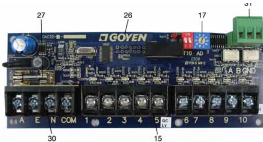
Figure 7: PS-LA AC output Large Terminal Expansion Card
