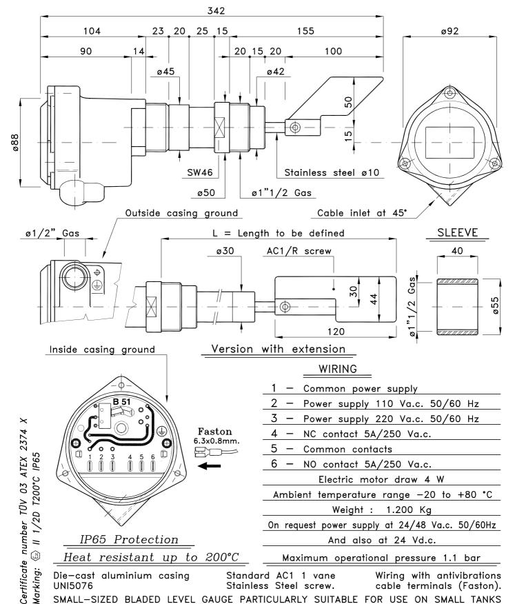
Die-cast aluminium casing UNI5076
