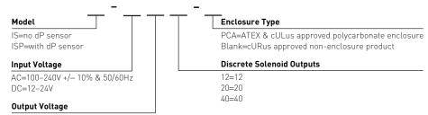
AC=same as AC input (100–240V +/– 10% & 50.60Hz) DC=same as DC input (12–24V DC),
